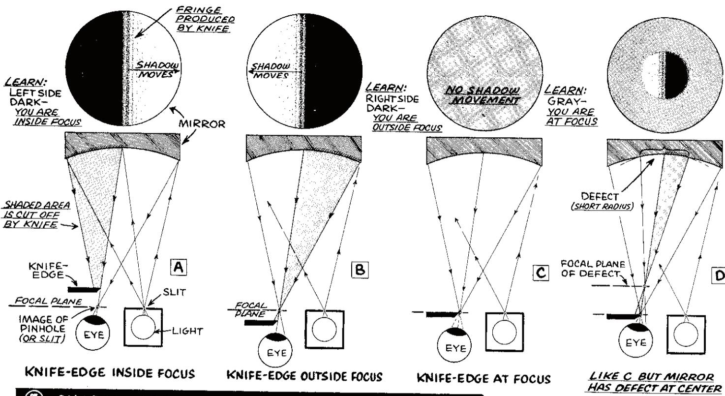
**⑤ SHADOW APPEARANCE OF A SPHERICAL MIRROR**
