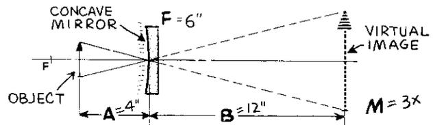
WHEN THE OBJECT-TO-LENS DISTANCE IS LESS THAN  $F$ , THE IMAGE IS VIRTUAL, ERECT AND MAGNIFIED.  $M$  IS NEVER LESS THAN  $1x$ ... IS GREATEST WHEN OBJECT IS JUST INSIDE  $F$ .
