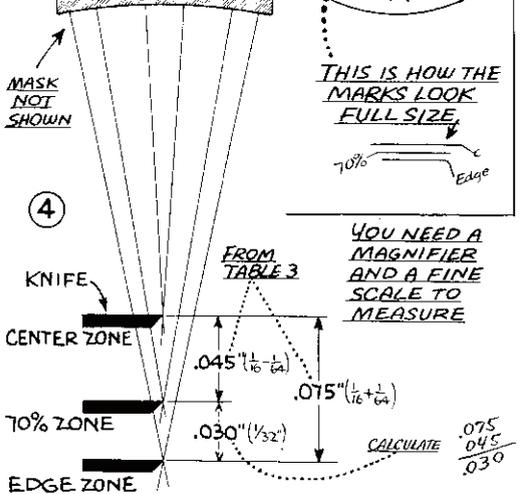
PARABOLA, SPHERE, DEEPEN?, INSTRUCTIONS: DEEPEN THE CENTER OF THE SPHERE TO MAKE A PARABOLA.
