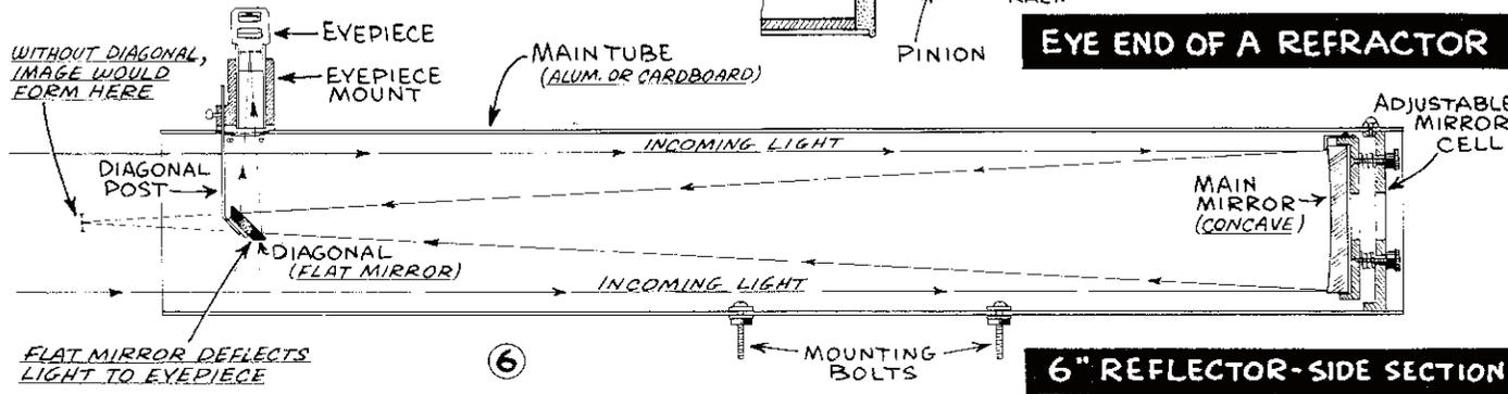
(2) its closed tube means cleaner optics and less air disturbance within the tube, (3) it can be made nearly 100% glare-proof.
