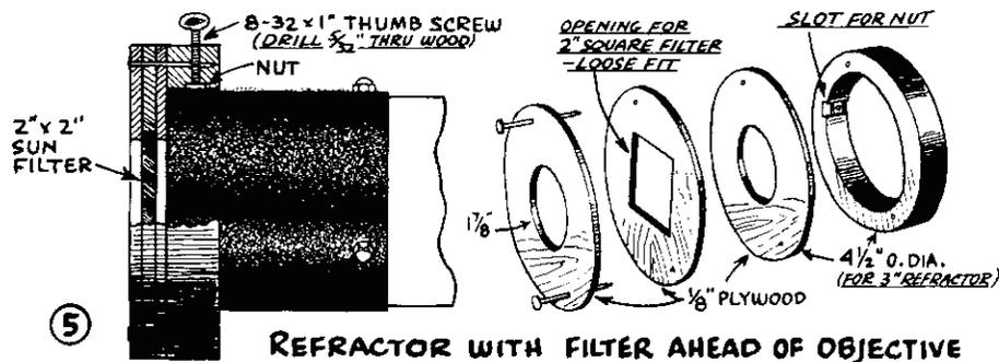
⑤ REFRACTOR WITH FILTER AHEAD OF OBJECTIVE
