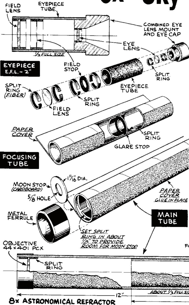
EDMUND simple lens telescope kit includes all the glass and parts to make an 8X astronomical refractor telescope. Of course the simple lens objective will show some false color and the image sharpness is not the best. However, the scope is good enough to show craters on the moon in sharp detail, and it will reveal hundreds of stars not visible to the naked eye.
