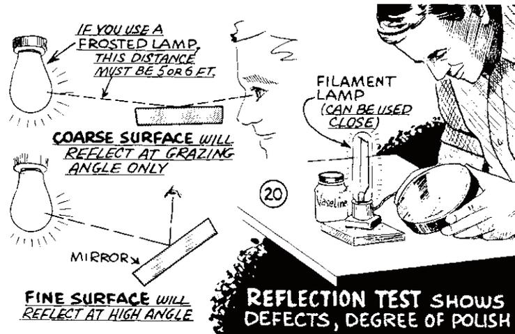
**REFLECTION TEST SHOWS DEFECTS, DEGREE OF POLISH**
