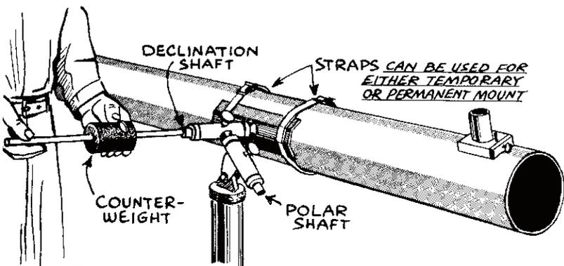
ORDINARY balancing of a telescope is a simple matter. You put the main tube in a horizontal position, Fig. 1, checking to see that both lock knobs are loose. The telescope is then balanced by moving the counterweight in or out as needed. Any slight imbalance can be remedied by applying moderate tension with the lock knobs; too much imbalance will cause an erratic action, particularly noticeable with a clock drive.
