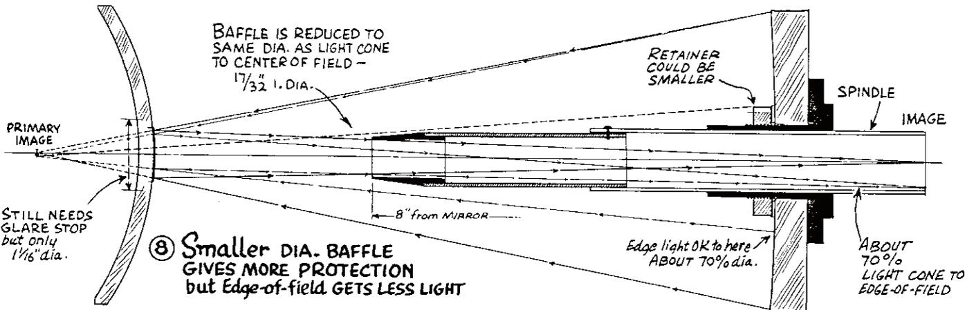
when properly installed. If you are buying a finished compound telescope of any kind, it is always wise to remove the eyepiece and look through the instrument. You should see only the secondary or its mounting; if you see "daylight" around the secondary or its mounting, you have a plain case of glare light. A little of this can be tolerated for astro use, but for the daytime scene you have to go all the way with 100% baffling of light outside the field of view.
