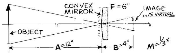
THE IMAGE IS ALWAYS VIRTUAL, ERECT AND REDUCED. B IS ALWAYS LESS THAN A, AND ALSO LESS THAN F. M IS ALWAYS UNDER 1X. WHEN THE OBJECT IS AT INFINITY, THE EQUATIONS BECOME USELESS AND UNNECESSARY. IN SUCH CASE:
