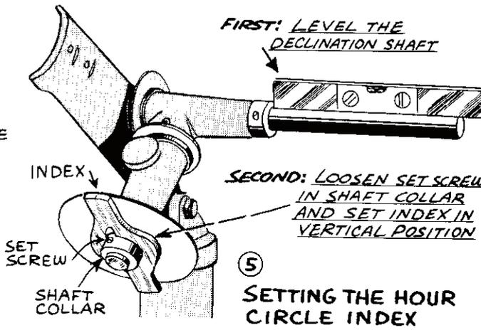
preferable because it calls for just one pointer which is always at the same fixed location. If a fixed circle is used, as in Fig. 6, it is best to have an index on both sides of the cradle to permit comfortable viewing at all positions of the telescope.
