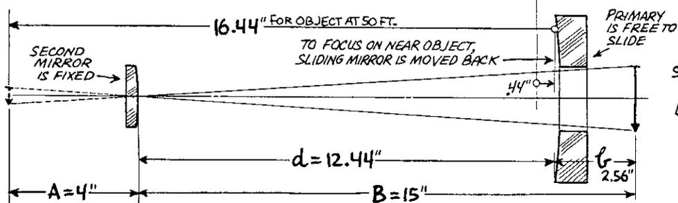
**C Constant Image Plane** IS OBTAINED BY SLIDING MIRROR... image always in same position for any distance
