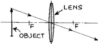
**Rule 2:** A LIGHT RAY PARALLEL WITH AXIS WILL, AFTER REFRACTION, PASS THROUGH THE REAR FOCAL POINT
