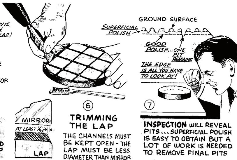
face sparsely charged. Each wet of rouge should be worked nearly dry since it is in this state that the rouge begins to wipe the glass with a vigorous polishing action. The drying mirror will become harder to push, and when it starts to stick and skip, it is time for a new charge of rouge. Polishing periods should be no less than 30 minutes--best to go an hour or more to get the frictional heat needed to allow the mirror to bed down snugly on its pitch pad.
