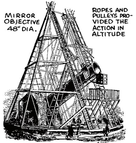
1789 HERSCHEL'S 40-FOOT REFLECTOR HAD A TILTED MIRROR TO PERMIT OBSERVING FROM FRONT OF TUBE. THE MOUNT ITSELF WAS AN ALTAZIMUTH
