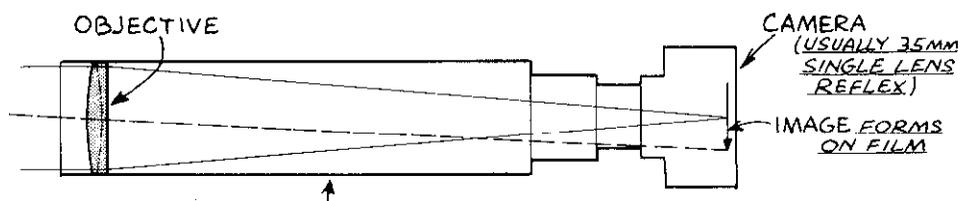
**2 AFOCAL** CONSISTS OF A TELESCOPE IN FOCUS AS FOR EYE USE, COMBINED WITH ANY CAMERA WITH LENS SET AT INFINITY
