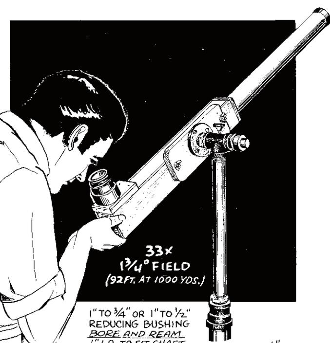
THIS is a neat prismatic telescope, only fairly bright because of the rather small objective, but clean and sharp over a wide field. The image is erect; you can use this scope day or night.
