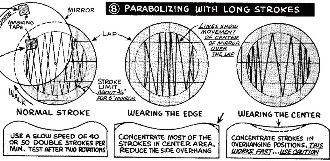
**LONG STROKE PARABOLIZING.** The actual work of parabolizing from a sphere or near-sphere is done with a stroke of maximum length and sidewise zig-zag, Fig. 8. Under good conditions you can parabolize a 6-inch f/8 in as little as five minutes. However, it is best to stretch the work over a longer period of about 20 minutes, using a slightly shorter stroke and less side overhang.
