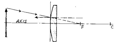
THE INTERSECTION OF ANY TWO RAYS WILL LOCATE THE IMAGE POSITION
