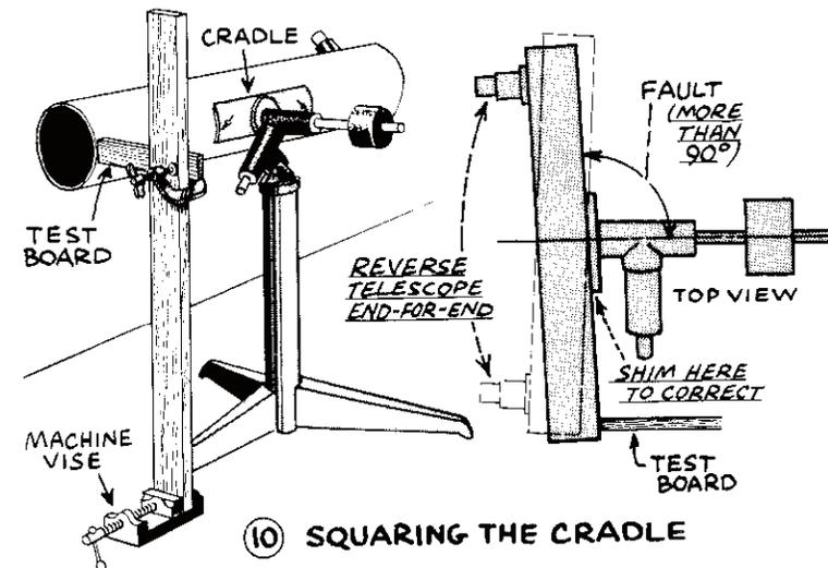
the declination shaft and the mounted telescope tube, seldom exceeding 1/4 degree. This can be corrected by placing cardboard shims between the cradle and main tube. A simple testing method is shown in Fig. 10. Reversing the main tube end-for-end, you will be able to detect a contact difference as small as 1/32 inch, which means about 5 min. of arc accuracy. This is close enough for a preliminary adjustment.
