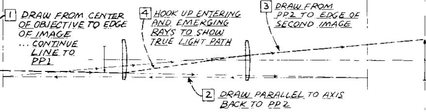
**ERECTOR M. SHOULD BE BETWEEN 1x AND 1.8x**
