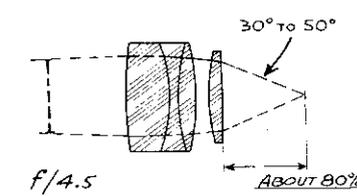
**ORTHOSCOPIC - FULLY CORRECTED FOR DISTORTION. WHEN MADE PROPERLY IT RATES AS BEST ASTRO EYEPIECE FOR HIGH POWER**
