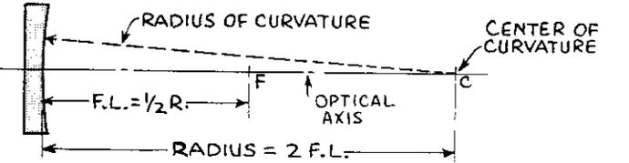
**1 GENERAL CASE - ALL MIRRORS:** THE FOCAL LENGTH OF A MIRROR = 1/2 THE RADIUS OF CURVATURE
