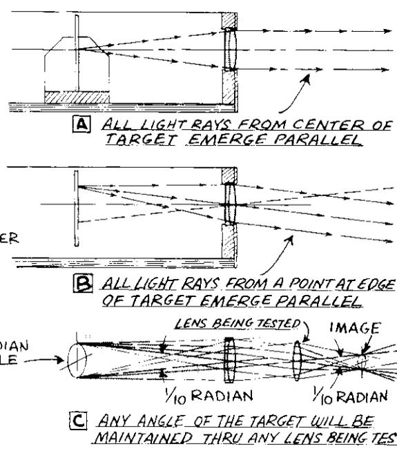
fine for riflescopes, finderscopes and small terrestrial and astro telescopes. Suitable equipment to test a 6-inch reflector is somewhat of an over-size luxury. However, you can do many tests and operations with a small collimator.
