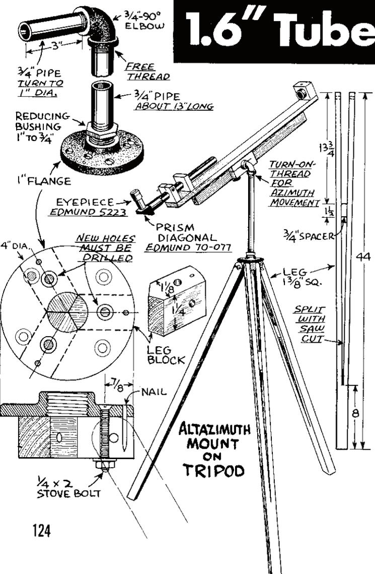
IF YOU want a cheap but good small refractor, you will like this tubeless job. Used with a 28mm eyepiece (Edmund No. 5223) it magnifies 38X over a 2-1/2-moon field. A tubeless telescope of this kind is practical for astro work if shielded from outside light. Obviously, it is not much of a trick to span a light cardboard tube between objective and focusing tube block if you want to make use of the scope for day objects.
