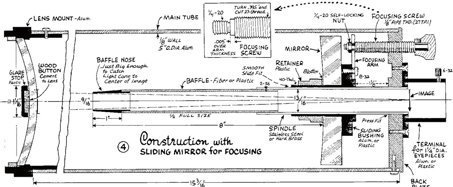
④ Construction with SLIDING MIRROR for FOCUSING
