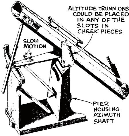
1722 HADLEY'S 6" REFLECTOR with PARABOLIZED MIRROR WAS MOUNTED ON A NEAT ALTAZIMUTH MOUNT. SLOW-MOTION WAS OBTAINED BY STRINGS WOUND ON PEGS
