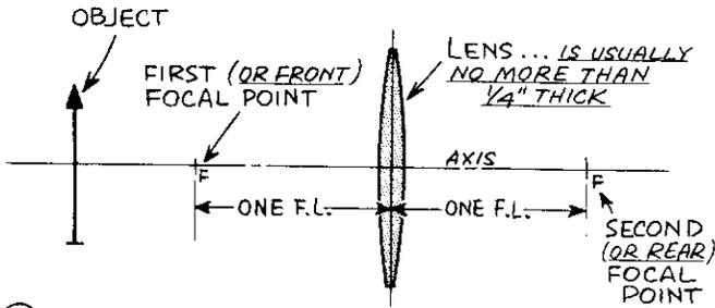
ONE WAY of solving the various object-image problems in optical design is to make an accurate drawing of the system to scale, after which you can run in the needed light rays graphically by following a few simple rules.
