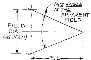
MEASURE THE ANGLE WITH A PROTRACTOR OR ADJUSTABLE TRIANGLE
