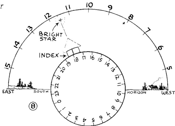
**at Start** THE HOUR CIRCLE IS IN ANY CHANCE POSITION. THE MOVING INDEX POINTS IN SAME DIRECTION AS TELESCOPE. THE INDEX SETTING IS A PERMANENT ADJUSTMENT... SEE OPPOSITE PAGE
