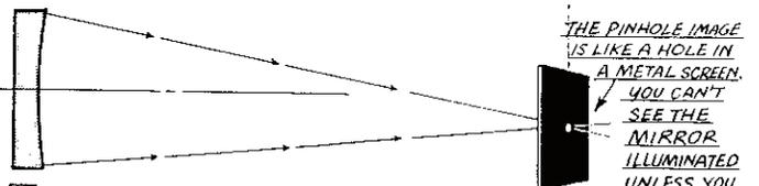
**6** THE IMAGE OF ANY APERTURE IS AS REAL, OPTICALLY, AS THE APERTURE ITSELF
