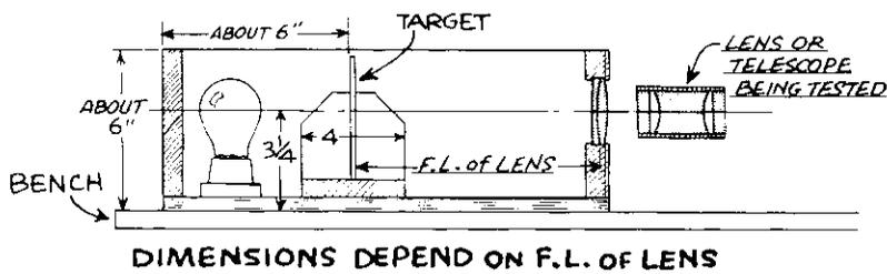
**④ BENCH COLLIMATOR and TARGET**
