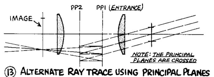
principal planes of the eyepiece as a whole and then draw light rays to the PP's, ignoring the lenses entirely except for the single item of diameter. The method of finding the PP's has already been described; the manner of making the drawing is as shown in Fig. 13. You draw a light ray to the image and keep right on going until you strike PP1. From PP1 to PP2, the ray is parallel to the axis. From PP2, the light ray goes to the corresponding part of the objective image, i.e., the exit pupil.
