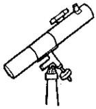
PRACTICALLY all of the early mounts were altazimuths. Such a mount has a primary axis in a vertical position, while the branch or secondary axis is horizontal. Movement around the primary axis moves the telescope to the right or left, technically known as a movement in azimuth; movement around the horizontal secondary axis moves the telescope up or down in altitude.
