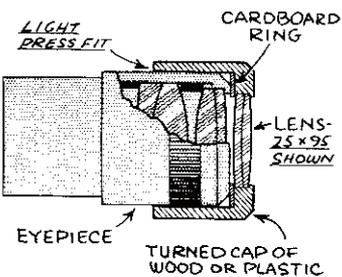
If you have an eyepiece with a good amount of eye relief, it is easy to boost the power as much as 40% by adding an extra lens, which is used as a cap over the eyepiece, as shown. The extra lens should be kept as close to the eyepiece as possible, and can face curved side in or out as desired. The shortened eye relief is still enough for comfortable use.
