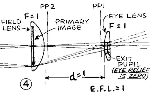
1-1-1 RAMSDEN IS CORRECTED FOR LATERAL COLOR BUT EYE RELIEF IS ZERO... DUST CAN BE SEEN ON FIELD LENS WHICH COINCIDES WITH IMAGE PLANE
