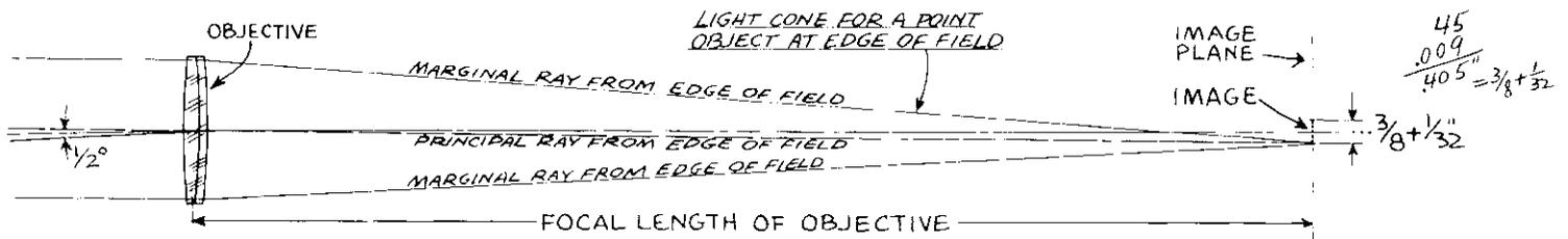
④ MINIMUM FULLY ILLUMINATED FIELD =  $\frac{1}{2}^\circ = \text{F.L.} \times .009$  Example: 3" f/15 REFRACTOR
