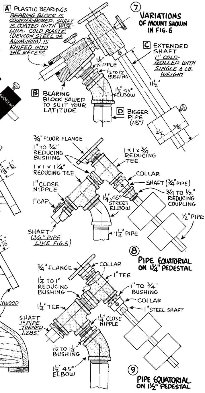
The only difficult part of making a pipe equatorial is the boring job, the 4 or 5-inch depth being near maximum for average home workshop equipment. An alternate is to rough-bore the bearings separately about .015 inch undersize, after which the assembly is made and the bearings hand reamed straight through to exact fit. Here again the required depth of cut is near the limit for ordinary reamers.
