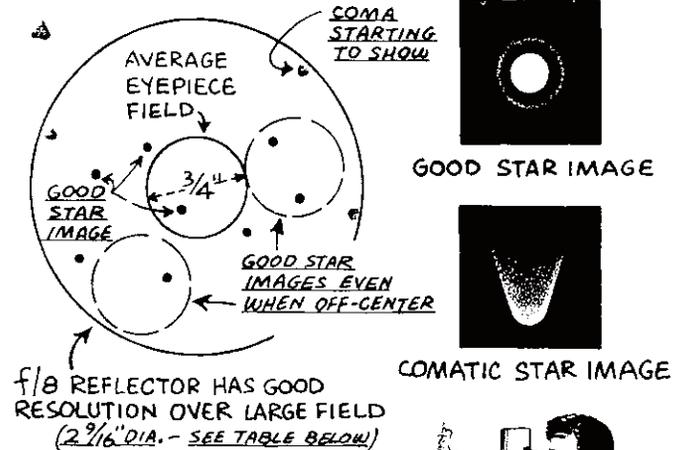
**Permissible "GOOD FIELD" for PARABOLIC MIRRORS**
