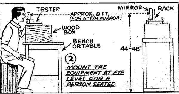
**MOUNT THE EQUIPMENT AT EYE LEVEL FOR A PERSON SEATED.**
