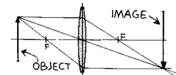
AFTER LOCATING THE IMAGE, YOU CAN "HOOK-UP" ANY NUMBER OF EXTRA RAYS. THE KEY RAYS FOR A SECOND LENS ARE EASILY LOCATED IN THIS MANNER, AFTER WHICH THE FINAL IMAGE IS LOCATED AS BEFORE
