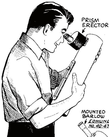
**YOU CAN HAND-HOLD AT 16x TO VIEW 3° ERECT FIELD... WITH BARLOW AND 1/2" EYEPIECE YOU GET 72x**
