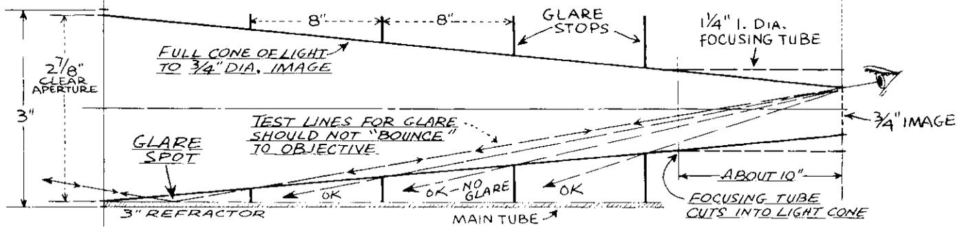
⑥ CONDENSED HORIZONTAL SCALE IS CONVENIENT WAY TO DRAW LIGHT CONE
