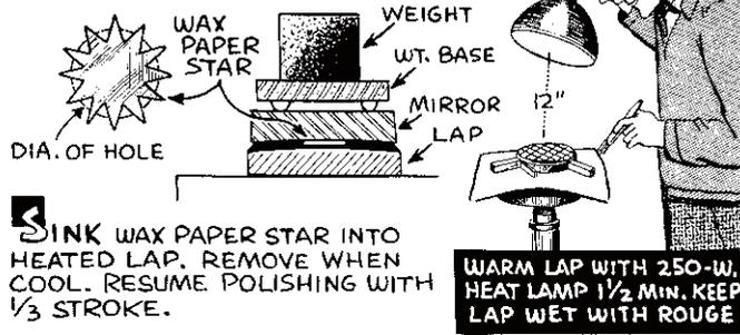
**ALTERNATE:** SCRATCHING, SANDING SHAVING OR FILING AT CENTER OF LAP. NO HEAT
