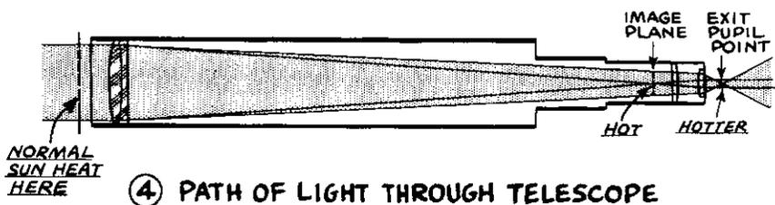
④ PATH OF LIGHT THROUGH TELESCOPE
