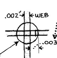
YOU KNOW THICKNESS OF RETICLE CROSS-HAIRS (WEB) AND WITH THIS AS GUIDE YOU CAN MAKE OUT-OF-FOCUS GUIDE STAR IMAGE THE PROPER SIZE
