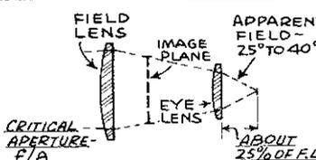
**HUYGENS - FIRST TWO LENS EYEPIECE. FULLY CORRECTED FOR LATERAL COLOR. DEFINITION IS GOOD, ESPECIALLY AT CENTER**
