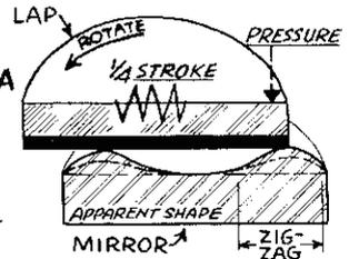
**RING Defects...** ARE SOMETIMES CAUSED BY LAP FAULTS. DIRT OR ABRASIVE ON A FACET WILL WEAR A DEPRESSED RING ON THE MIRROR SURFACE
