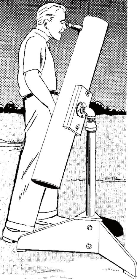
IF YOU are building a reflector on a tight budget, the best plan is to use top quality optics and save what you can on the mount and homemade parts. The result will be something like the design shown with simple turn-on-threads altazimuth mount and slide focusing. You will find this scope solid and satisfying, especially if it is a first instrument.
