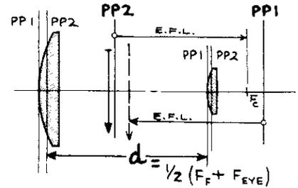
**SPACING:** LATERAL COLOR IN ANY SIMPLE EYEPIECE IS CORRECTED BY SPACING OF 1/2 THE COMBINED FOCAL LENGTHS. (LONGITUDINAL COLOR IS NOT CORRECTED). SPACING IS MEASURED BETWEEN ADJACENT PRINCIPAL PLANES
