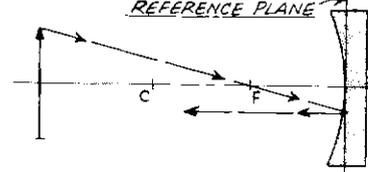
THE INTERSECTION OF ANY TWO OF THE THREE RAYS SHOWN WILL LOCATE THE POSITION OF IMAGE
