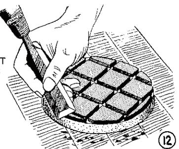
**TRIM THE LAP WITH A WOOD CHISEL OR RAZOR BLADE. INCLINE THE EDGE A LITTLE TO MAKE LAP ABOUT 1/16" LESS THAN MIRROR DIAMETER**
