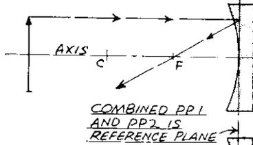
**Rule 3:** A RAY PASSING THRU THE FOCAL POINT WILL BE REFLECTED PARALLEL TO AXIS
