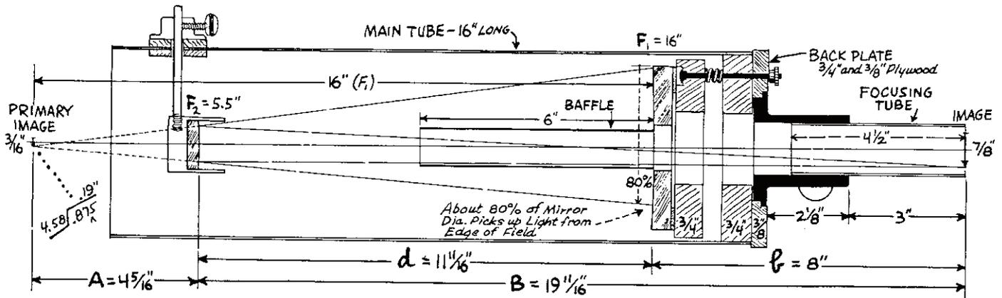
**STAR DIAGONAL** - With FIXED OPTICS, A LONG "f" DISTANCE IS NEEDED, USING RACK-and-PIION FOCUSING
