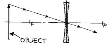
**Rule 2:** A LIGHT RAY PARALLEL TO THE AXIS WILL, AFTER REFRACTION, APPEAR TO COME FROM THE FRONT FOCAL POINT
