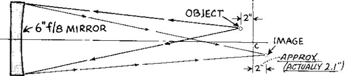
**4** IF THE OBJECT IS MOVED A SHORT DISTANCE TOWARD MIRROR, THE IMAGE WILL MOVE A SHORT DISTANCE AWAY FROM MIRROR
