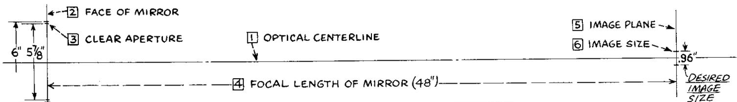
**OPTICAL LAYOUT for ANY NEWTONIAN REFLECTOR**
