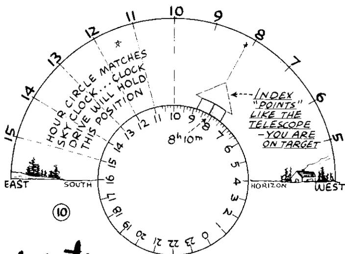
**Operation 2** SLIP-TURN THE HOUR CIRCLE TO PUT R.A. OF PILOT STAR (11<sup>h</sup> 30<sup>m</sup>) IN LINE WITH THE INDEX. NOTE THE HOUR CIRCLE NOW MATCHES THE SKY CLOCK
