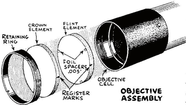
THE REFRACTOR is an easy scope to build, especially when you buy the main parts readymade. Then, the only problem is how long to make the main tube in order to have enough focusing adjustment for a camera, star diagonal, Barlow lens, etc. This plan specifies 35-1/2 inches long for the main tube and this length combined with an extension focusing tube will give you a 10-inch focusing range--enough for almost any attachment except possibly a very long Porro prism erector.
