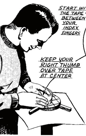
**8 PARABOLIZING WITH LONG STROKES**
