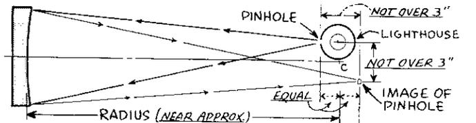
**5 USUAL SETUP FOR TESTING.** PINHOLE IMAGE AT REAR OF LIGHT IS CONVENIENTLY PLACED FOR OBSERVATION. THE SMALL DISPLACEMENTS WILL NOT AFFECT IMAGE QUALITY OR MEASUREMENTS
