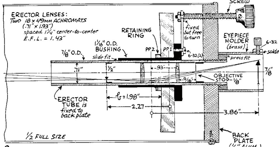
**CONSTRUCTION with SLIDING MIRROR FOCUS**
