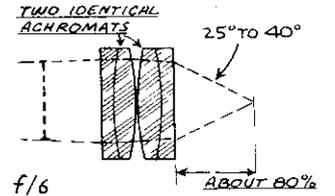
**SYMMETRICAL - A POPULAR HOMEMADE STYLE. FOCAL LENGTH IS ABOUT ONE-HALF F.L. OF LENSES USED... IS GOOD ASTRO EYEPIECE**
