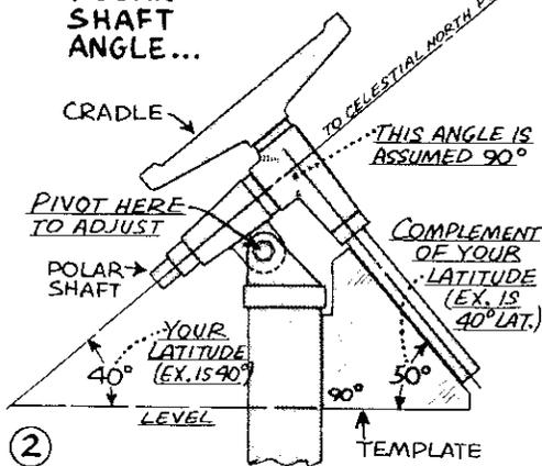
② ... IS SET IN A ROUNDABOUT WAY BY MEASURING THE TILT OF DECLINATION SHAFT
