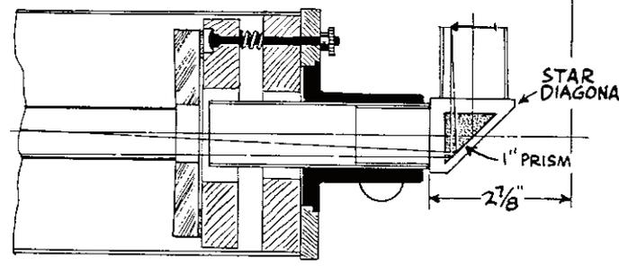
bit larger, specifically 5/32 inch for this design where the diameter of the image is 1/8 inch. With sliding primary, the extended erector tube is practically a full light baffle, making the objective stop less important but always worth fitting.
