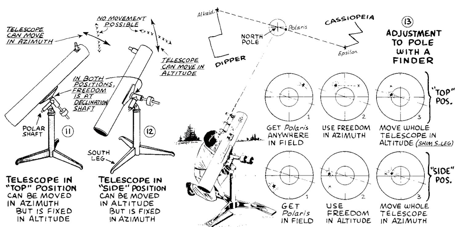
finderscope is much the same as with a bore-scope, except you have to do the sighting twice in order to eliminate the movement of the telescope itself.
