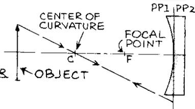
**Rule 2:** A RAY PARALLEL TO THE AXIS WILL BE REFLECTED THROUGH THE FOCAL POINT
