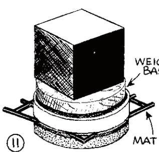
**PRESS WITH WEIGHT IF PITCH GETS TOO HARD FOR EASY FORMING. REHEAT THE WHOLE LAP IF NEEDED AS SHOWN AT TOP OF PAGE**
