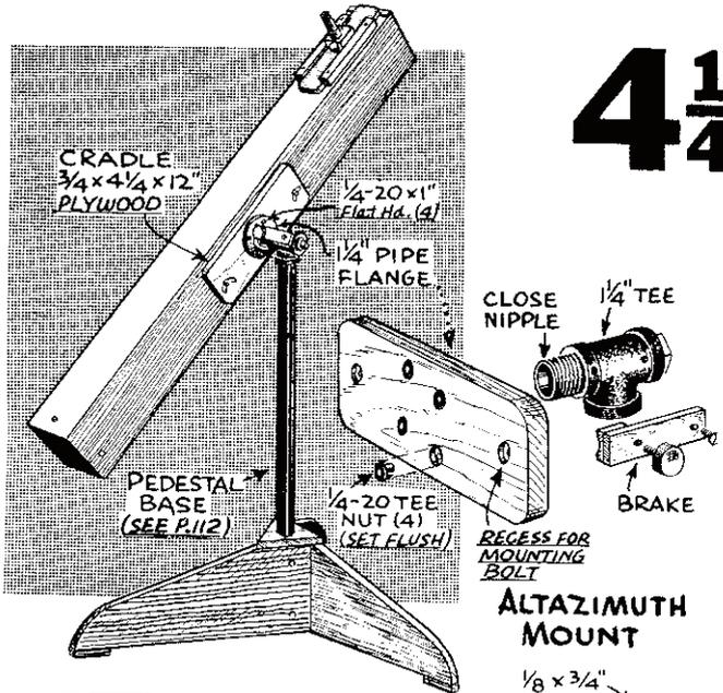
PLYWOOD TUBES are practical for telescopes, the main fault being that the common square shape is a bit more bulky than a round tube of cardboard or metal. A good feature is low heat conduction which means less air disturbance. The flat sides of the square tube are made-to-order for focusing devices working length-wise, such as the one shown. This permits 6 in. of travel--plenty for all eyepieces and most attachments.
