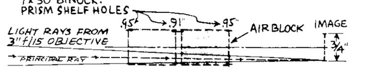
**15 LIGHT PATH - PRISMS SHOULD PASS AT LEAST THE PRINCIPAL RAY. EXAM DIP SHOWS WHOLE CONE GETS THRU**
