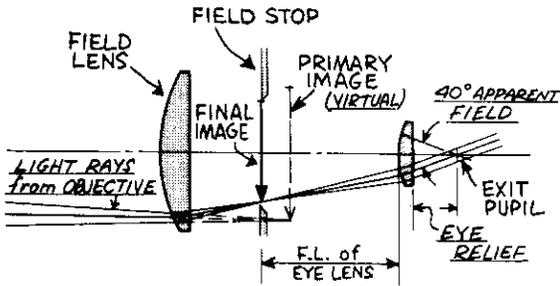
**LIGHT PATH:** WITHOUT EYEPIECE, THE TELESCOPE OBJECTIVE WOULD FORM PRIMARY IMAGE AS SHOWN. THE FIELD LENS INTERCEPTS THE LIGHT RAYS AND FORMS A REAL FINAL IMAGE WHICH IS VIEWED BY THE EYE LENS
