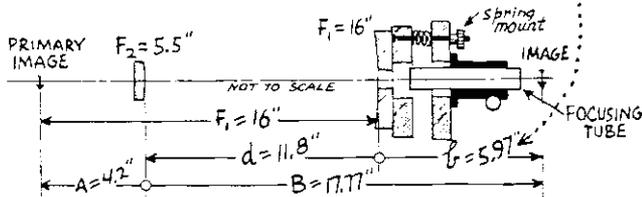
**BIG "l" NEEDED FOR Rack-and-pinion FOCUSING**
