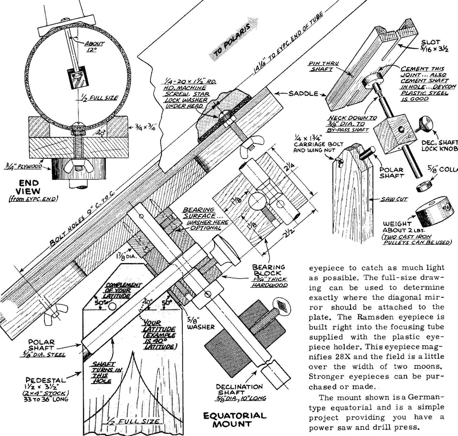
eyepiece to catch as much light as possible. The full-size drawing can be used to determine exactly where the diagonal mirror should be attached to the plate. The Ramsden eyepiece is built right into the focusing tube supplied with the plastic eyepiece holder. This eyepiece magnifies 28X and the field is a little over the width of two moons. Stronger eyepieces can be purchased or made.
