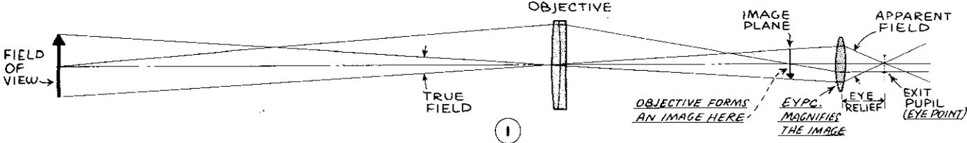
OPTICAL SYSTEM OF THE TELESCOPE
