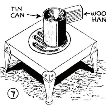
**MELT THE PITCH IN A TIN CAN... IT WILL MELT IN LESS THAN 10 MINUTES**
