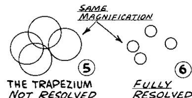
a light cone, and the brain gets the same impression as if the cone were fully illuminated. But the telescope has to magnify a star 13x per inch of objective diameter to fully illuminate one cone. Hence, even at the top magnification of 50x per inch, stars are magnified only about four times the naked-eye view.
