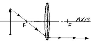
THE INTERSECTION OF ANY TWO OF THE THREE LIGHT RAYS SHOWN WILL LOCATE THE POSITION OF THE IMAGE
