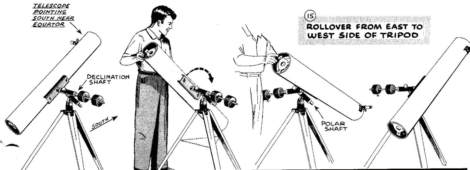
TELESCOPE EAST OF TRIPOD ...TILT FRONT OF TUBE DOWN ... ROLL OVER TO WEST SIDE ... ELEVATE THE TUBE
