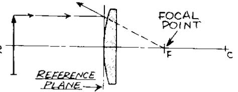
**Rule 3:** A RAY AIMED AT THE FOCAL POINT WILL BE REFLECTED PARALLEL TO AXIS. A BACKWARD EXTENSION OF THIS RAY WILL PASS THRU THE IMAGE POINT
