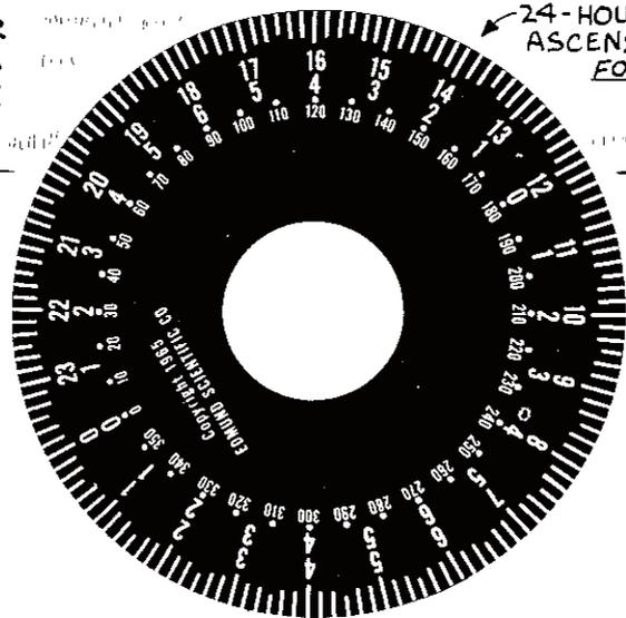
0-6-0-6 SCALE IS HOUR ANGLE SCALE
