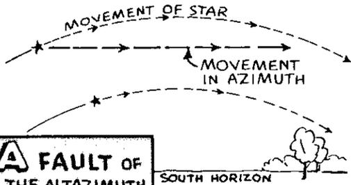
**A FAULT OF THE ALTAZIMUTH MOUNT IS THAT THE MOVEMENT IN AZIMUTH IS NOT THE SAME AS THE PATH OF A STAR**
