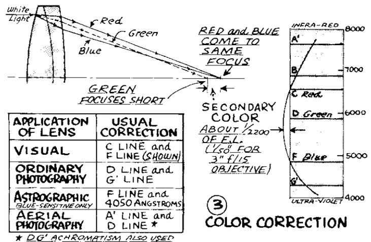
for use with infra-red and other red-sensitive emulsions. Such a glass is poor for visual use because the blue rays are badly out of focus.
