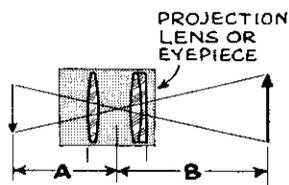
FOR DOUBLE LENSES OR ANY TYPE OF EYEPIECE, MEASURE FROM CENTER. THIS IS NOT EXACT BUT CAUSES NO GREAT ERROR, ESPECIALLY AS APPLIED TO DIMENSION "B"
