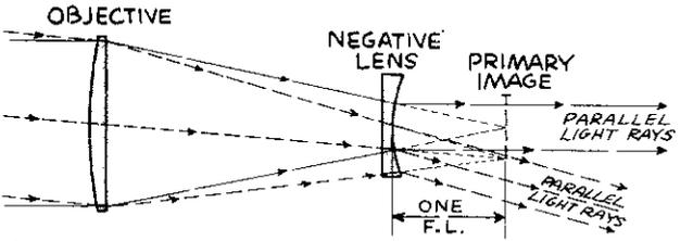
AFOCAL - EMERGENT RAYS DO NOT COME TO A FOCUS - NO IMAGE IS FORMED. THIS SPACING IS A GALILEAN TELESCOPE
