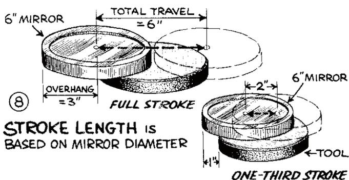
8 STROKE LENGTH IS BASED ON MIRROR DIAMETER
