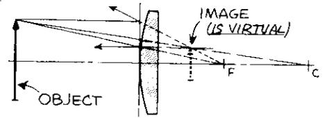
of an entering and emergent parallel ray gives this method its name. Fig. 4 explains the parallel ray method as applied to a negative lens, while Figs. 7 and 8 cover similar situations where a mirror is the optical element.
