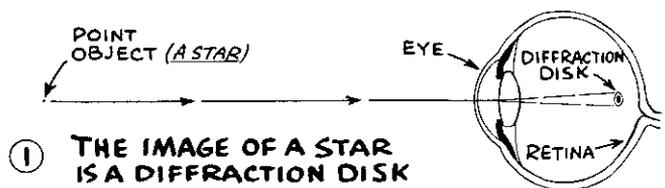
① THE IMAGE OF A STAR IS A DIFFRACTION DISK
