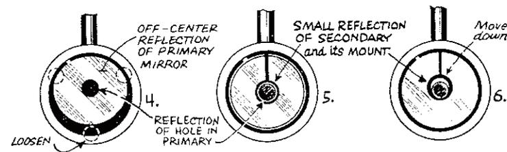
VERTICAL OFF-CENTERING IS CORRECTED BY TURNING BOTTOM ADJUSTING NUT
