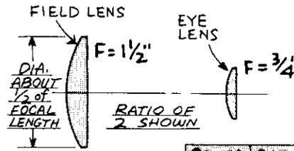
**RATIO:** FIELD LENS IS ALWAYS LONGER F.L. THAN EYE LENS. BEST RATIO DEPENDS ON POWER OF SCOPE AND SHOULD BE SELECTED FROM TABLE
