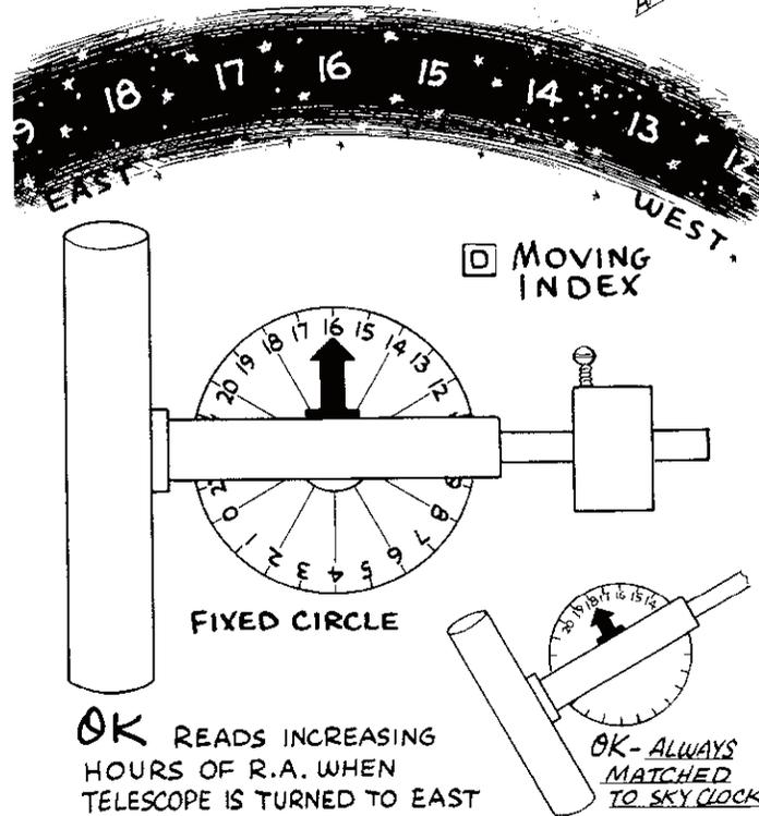
numbers on the hour circle would not match the imaginary clock in the sky. The other two systems do not work at all--they simply do not index or point the telescope the right way. However, even these arrangements can be used to set off an hour angle.
