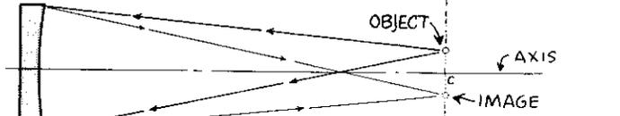
**3** IF THE OBJECT IS DISPLACED TO ONE SIDE OF THE AXIS, THE IMAGE WILL FORM AT SAME DISTANCE ON OPPOSITE SIDE
