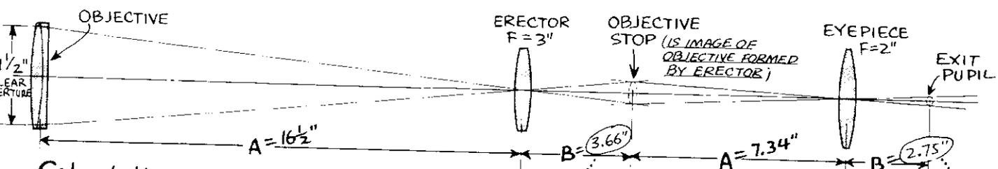
Calculation - OBJECTIVE STOP POSITION and DIAMETER
