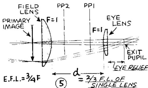
1-1-2/3 RAMSDEN IS STOCK DESIGN WITH LENSES SAME F.L. AND SPACE 2/3 F.L. OF SINGLE LENS. SPACING LESS THAN 1/2(F+F) CAUSES LATERAL COLOR
