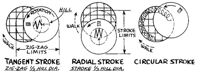
YOU CAN USE ANY OF THE THREE STROKES SHOWN WATCH THE TAPE! ANY OVERHANGING STROKE WITH MIRROR ON TOP MUST BE PACED BY THE MIRROR ROTATION - NOT THE WALK-AROUND. ALWAYS DO A WHOLE NUMBER OF ROTATIONS. TWO ROTATIONS WILL LEVEL A SMALL HILL
