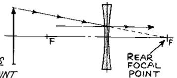
THE INTERSECTION OF ANY TWO OF THE THREE RAYS SHOWN WILL LOCATE THE POSITION OF THE IMAGE
