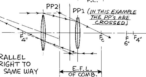
the principal planes are crossed, this means you must then backtrack to PP2, as can be seen in Fig. 10B example.
