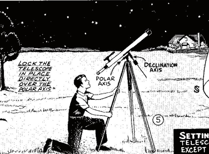
LOCK THE TELESCOPE IN PLACE DIRECTLY OVER THE POLAR AXIS
