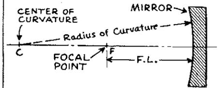
ALL TELESCOPE MIRRORS  $\left\{ \begin{array}{l} \text{F.L.} = \frac{1}{2} \text{ Radius} \\ \text{Radius} = 2 \times \text{F.L.} \end{array} \right.$
