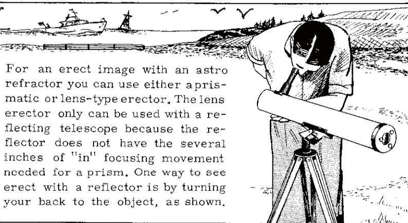
For an erect image with an astro refractor you can use either a prismatic or lens-type erector. The lens erector only can be used with a reflecting telescope because the reflector does not have the several inches of "in" focusing movement needed for a prism. One way to see erect with a reflector is by turning your back to the object, as shown.
