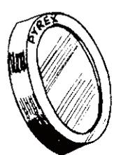
**PYREX** IS THE PREFERRED GLASS, CHIEFLY FROM ITS LOW EXPANSION WHICH IS ONLY 1/3 AS MUCH AS PLATE GLASS. THE BACK OF THE DISK IS (USUALLY) CLEAR, ALLOWING YOU TO SEE THE "ACTION" WHEN GRINDING AND POLISHING. IF YOU HAVE THE BAD LUCK OF EXPOSING A BUBBLE ON SURFACE, GO RIGHT AHEAD. PAINTED BLACK AFTER ALUMINIZING, IT WILL NOT HARM THE MIRROR.
