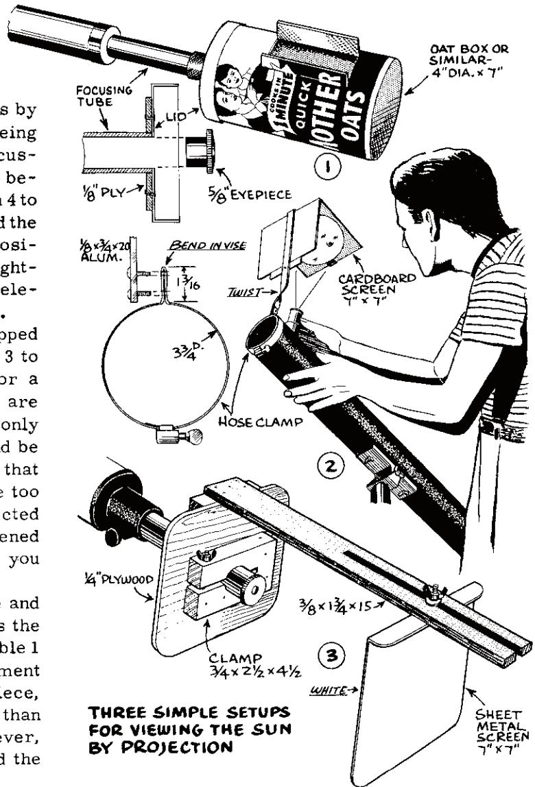
THREE SIMPLE SETUPS FOR VIEWING THE SUN BY PROJECTION
