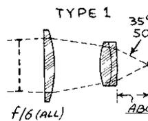
**KELLNER - BASIC FORM (TYPE 1) HAS ACHROMATIC EYE LENS FOR BETTER COLOR CORRECTION THAN RAMSDEN. TYPE 3 (PLOSSL) RATES WITH THE FINEST TELESCOPE EYEPIECES... IT OFFERS WIDE FIELD AND COMFORTABLE EYE RELIEF**
