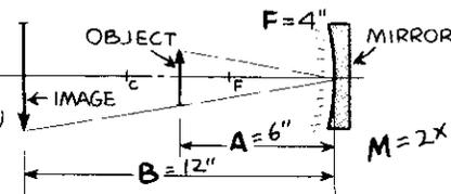
**TWO CASES:** WHEN THE OBJECT IS MORE THAN  $F$  BUT LESS THAN  $2F$  FROM LENS (SHOWN), THE SYSTEM IS PROJECTION-- THE IMAGE IS LARGER THAN OBJECT.
